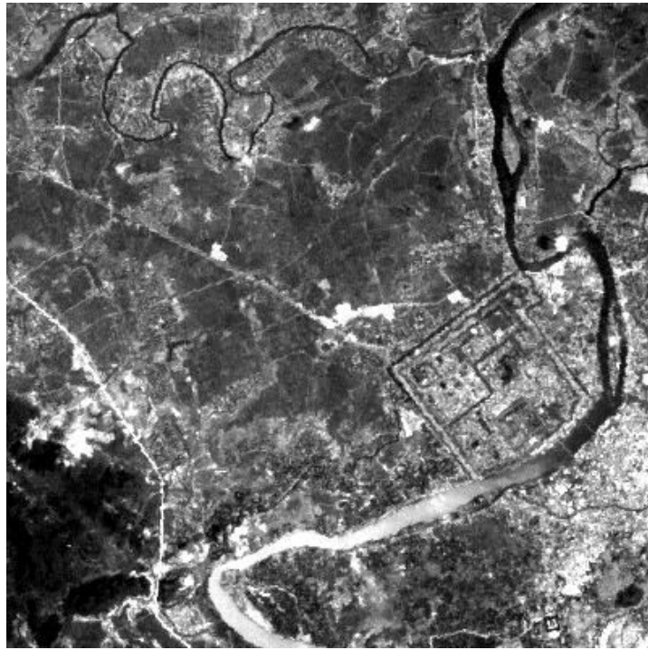
Landsat band 2 - (wavelength range = 0.52-0.60 \mu\text{m} = blue light)
