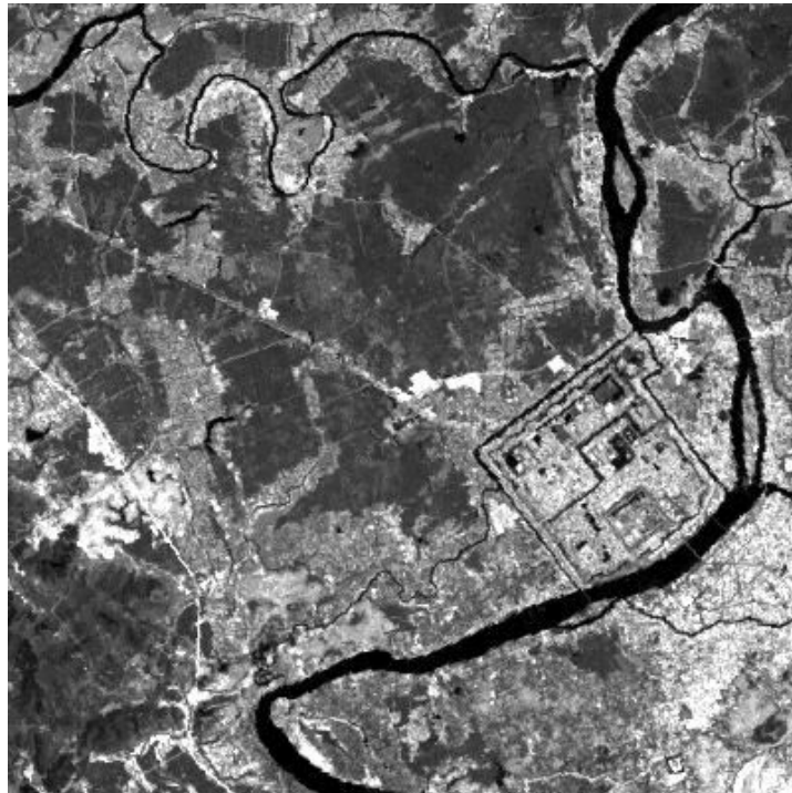
Landsat band 7 - (wavelength range = 2.08-2.35 \mu\text{m} = mid-infrared light)
