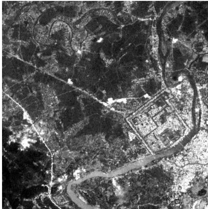
Landsat band 1 - (wavelength range = 0.45-0.52 \mu\text{m} = blue-green light)
