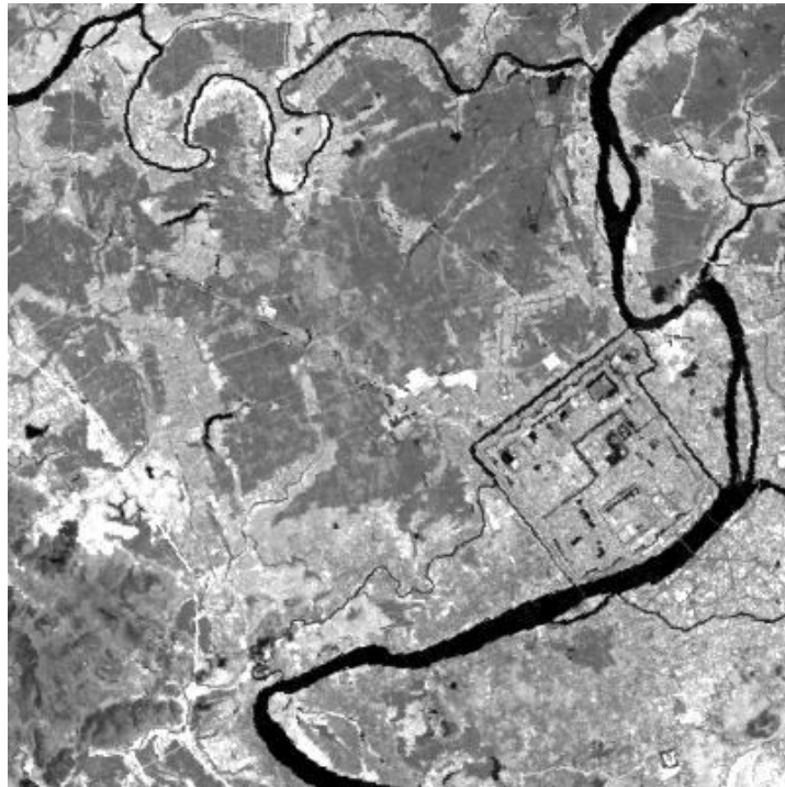
Landsat band 5 - (wavelength range = 1.55-1.75 \mu\text{m} = mid-infrared light)
