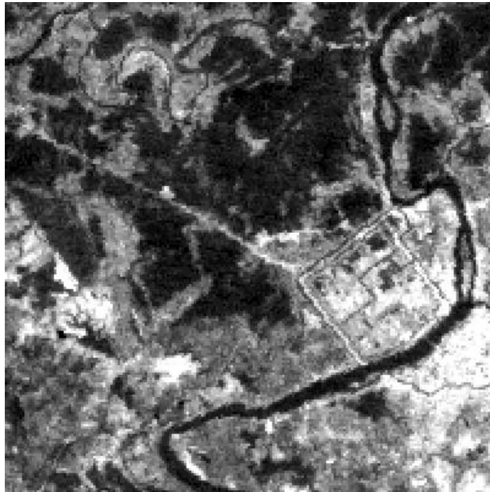
Landsat band 6 - (wavelength range = 10.40-12.50 \mu\text{m} = thermal-infrared light)
